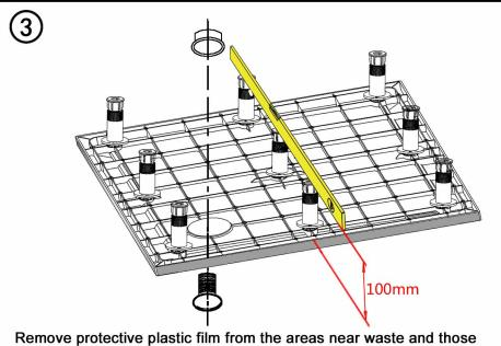
sides of the tray which will be against a wall. Fit the shower tray waste. all feet should be adjusted to 100mm.
